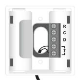
Remove the internal temperature sensor from the "T" terminal of the TA1 sensor. Connect the external temperature probe to the TA1 sensor's "T" terminal. 100' maximum distance.
