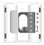
For installations where 3-wires already exist or can be run from a TS200(H) thermostat to the TA1 sensor. Mount the TA1 sensor directly on the wall. Connect TA1 sensor's D, C, and R terminals to matching terminals at TS200(H). 500' maximum distance.
