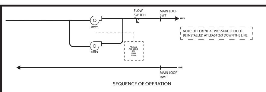
PM5 will be scheduled to start based on an occupied start time. Pump with lowest run-time will start. If flow is detected, pump will remain enabled until change-over timer (adjustable) is met, at which point secondary pump will be enabled. If flow is not detected when a pump is enabled, alarm will be generated at Pelican EMS and standby-pump will be enabled. If standby-pump does not generate flow a second alarm will be generated at Pelican EMS.
