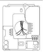
Use the included screws to attach the thermostat backplate to the wall. Follow one of the examples below:
